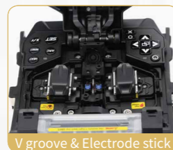
V groove & Electrode stick
